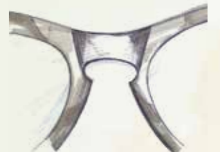
KEYHOLE BRIDGE Shaped like an old-fashioned keyhole, it fits only on the face sides without touching the top. This design element is created by a milling technique
